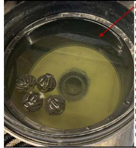
Inside the 5 gal bio pressure filter after a few minutes the coagulated diatoms and attached nutrients have fallen to the bottom of the filter leaving clear water above. The mass at the bottom is approx 9 cubic inches of material.
